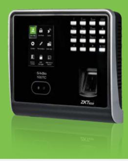
SilkBio-100TC is the first ever Time & Attendance and Access Control Terminal to be associated with SilkID fingerprint reader, face recognition and FRID card functions. With the new SilkID fingerprint reader, the operation remain stable under strong light source and high preciseness of verification of wet and rough fingers. With latest facial algorithm and the innovation features, Silkbio-100TC is bringing you the whole new experience.
